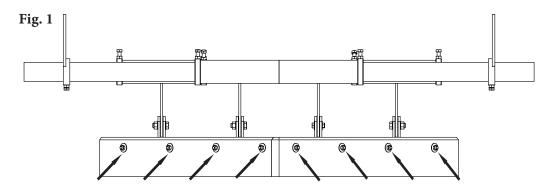
3. Test run and inspect. Run the belt and check that the Twin Pole V-Plough runs smoothly and has an effective cleaning action. If any vibration occurs, turn the adjuster to raise the nose slightly.
